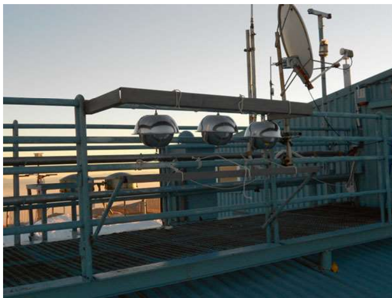
Photograph 24.2 Passive air samplers at BEO Moussala
